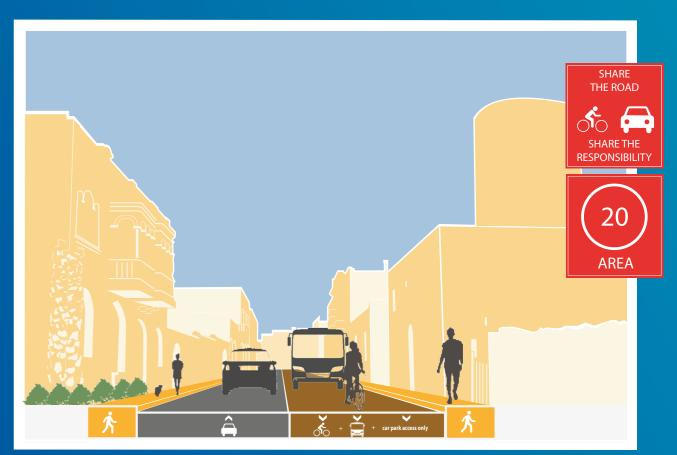
To better alert drivers of the road section which drastically narrows down (the stretch of road between Triq il-Viżitazzjoni and Triq Dun Alwig Mizzi), tactical urbanism is being proposed in the form of colourful markings. In addition, adequate signage is also being proposed for limited access, sharing of road and further slow speed signs.
